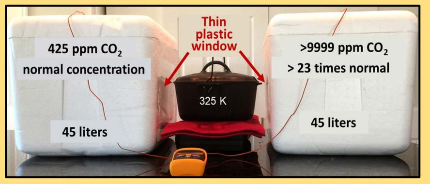
When measuring the increase in temperature of air caused by infrared radiation from a black body at 325K (125°F), there was no difference, within the resolution of the digital thermometer (0.1K), between the temperature of normal air and of air containing >23 times normal concentrations of  $CO_2$ .
