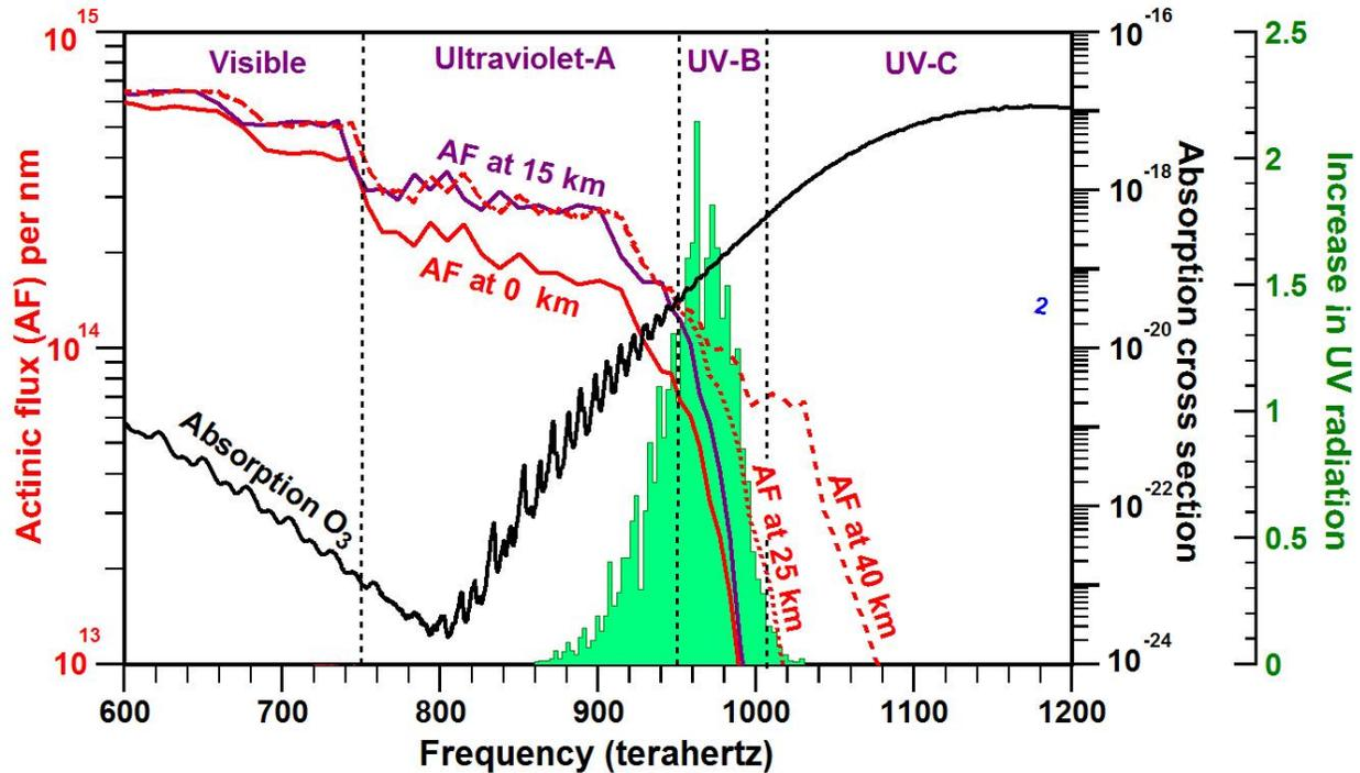
Figure 7. Percent increase in ultraviolet radiation (green) reaching the lower troposphere when the ozone layer is depleted by 1%. These frequencies between 900 and 1000 THz are the most energetic solar radiation to reach Earth.
