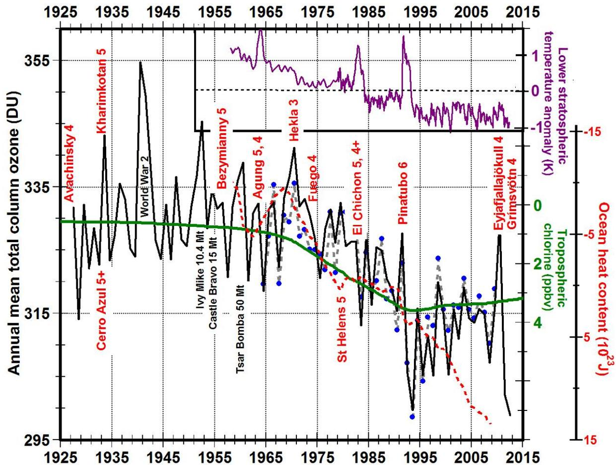
Figure 8. Mean annual total column ozone above Arosa, Switzerland (black line), anthropogenic tropospheric chlorine (green line), ocean heat content (dashed red line) and lower stratospheric temperature anomaly (purple line). Note that the y axes of the green and dashed red lines are inverted. The dashed gray line with blue data markers shows, for 1964 to 2009, the annual mean area-weighted total ozone deviation from the 1964 to 1980 means for northern mid-latitudes.
