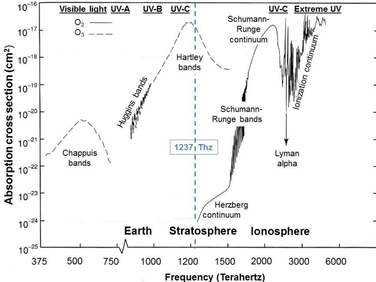
Figure 6. The amount of absorption of solar radiation by oxygen (solid lines) and by ozone (dashed lines) as a function of frequency is low in the Herzberg continuum, just to the right of the 1237 THz blue dashed line, explaining the minimal absorption by an altitude of 20 km between 1350 and 1600 THz shown in Figure 5. Replotted as a function of frequency from Figure 3.5 of *Liou* [2002].
