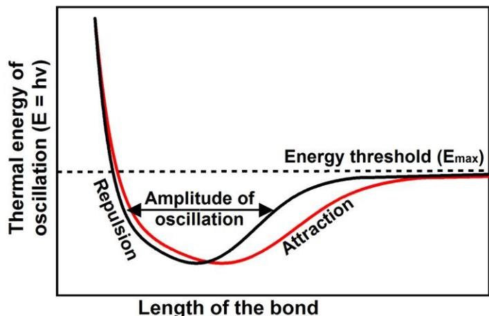
Figure 1. The length of each bond holding matter together oscillates between electrodynamic forces of repulsion on the left and electrodynamic forces of attraction on the right. When energy equals or is greater than the threshold energy ( $E_{max}$ ) the bond comes apart. At a higher temperature, the length of the bond increases and the amplitude of oscillation at every frequency increases (red line).
