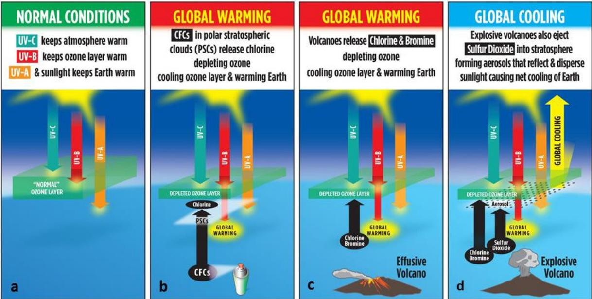
Figure 9. a) Conditions normal before 1965. b) CFCs release atoms of chlorine that deplete the ozone layer allowing more UV-B to reach Earth. c) Effusive volcanoes emit chlorine and bromine, which deplete ozone, leading to global warming. d) Explosive volcanoes similarly deplete ozone, but form globe-encircling aerosols that reflect, scatter, and absorb solar radiation, causing net global cooling.
