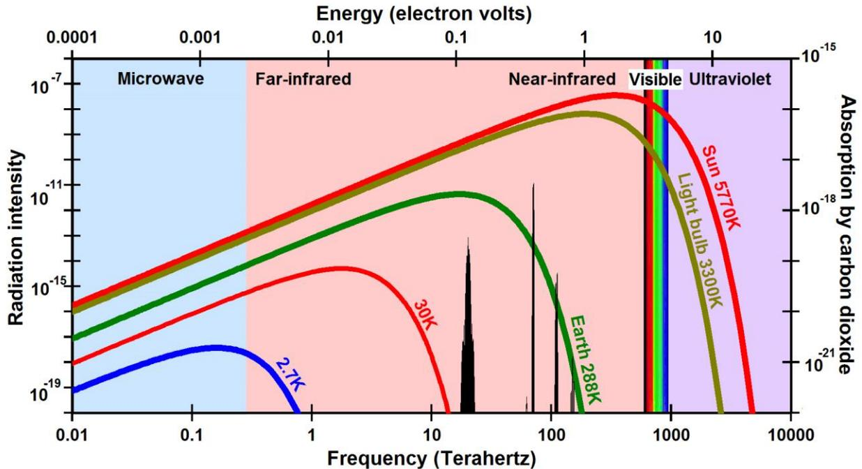
Figure 2. Planck's law calculates the intensity of radiation at each frequency of oscillation as a function of the temperature in Kelvin of a black body at thermal equilibrium.
