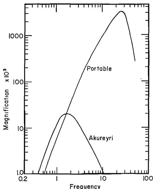
Fig. 2. Ground amplitude magnification of the suitcase seismograph used in this study assuming the lower geophone sensitivity (see text). The magnification of the World-Wide Standardized Seismic Network short-period instrument at Akureyri is shown for comparison.
