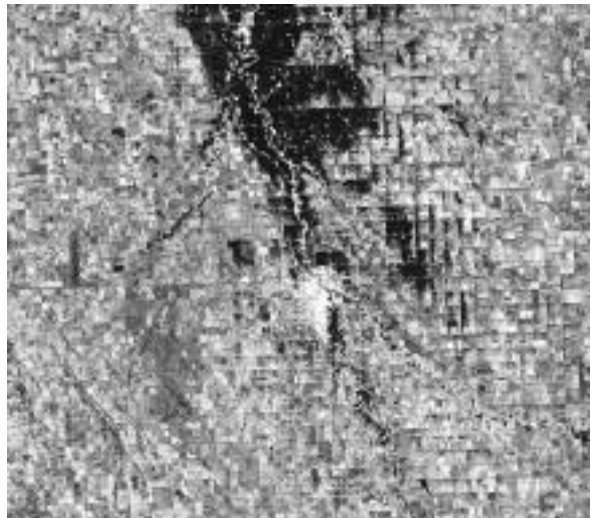
RADARSAT image of the extent of flooding in Grand Forks, ND, during the 1997 Red River floods.
