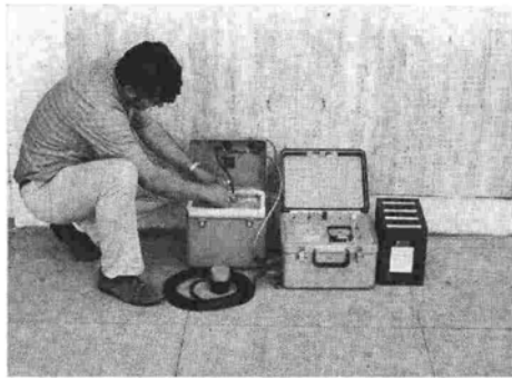
FIG. 2 - Demonstration set-up of transmitter for sending data to the satellite (left), multi-level seismic counter (center), and one year's supply of batteries (right). Except for geophone (left, front) and transmitter antenna (not shown), components are placed in a metal box for transportation and semi-permanent field installation.
