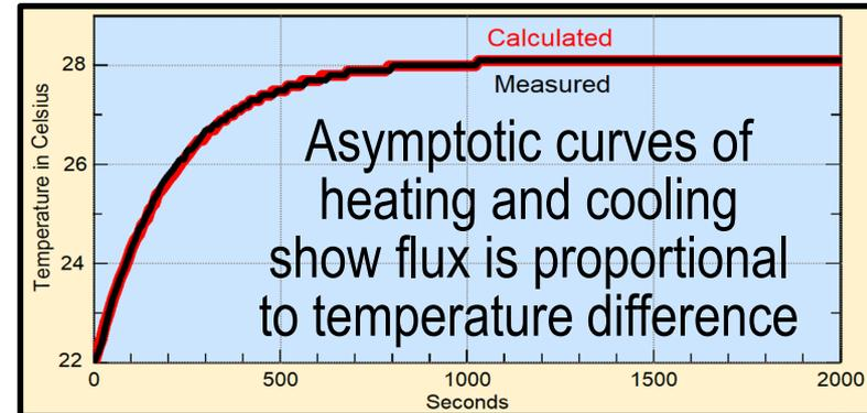
The measured black curve is the warming caused by a picture light shining on a small black piece of metal. The calculated red curve is the temperature calculated by multiplying 4.6% times the average of the existing temperature and the ending temperature of 28 °C at each 10-second interval. The 4.6% has to do with the conductivity per second of heat into the black object and other boundary conditions.
