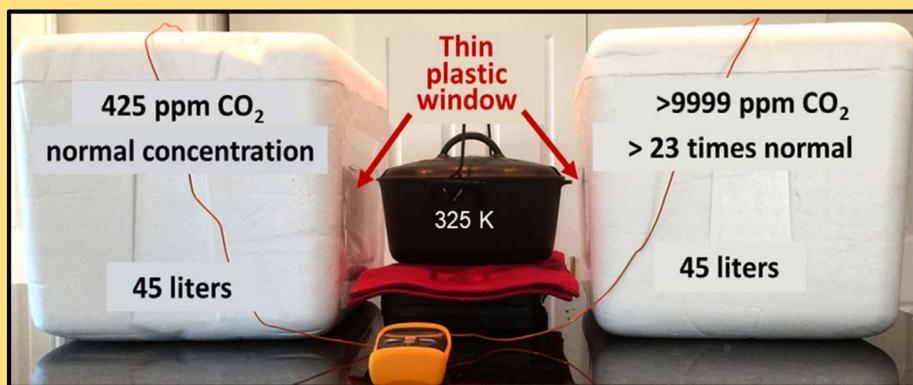
When measuring the increase in temperature of air caused by infrared radiation from a black body at 325K (125°F), there was no difference, within the resolution of the digital thermometer (0.1K), between the temperature of normal air and of air containing >23 times normal concentrations of CO<sub>2</sub>.
