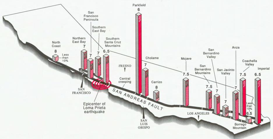
The probability of major earthquakes occurring between 1988 and 2018 is shown for segments of four major faults in California; these probabilities were determined 1 year before the Loma Prieta earthquake and are currently being reevaluated. The expected magnitude for an earthquake on each segment is shown above each box. The height
