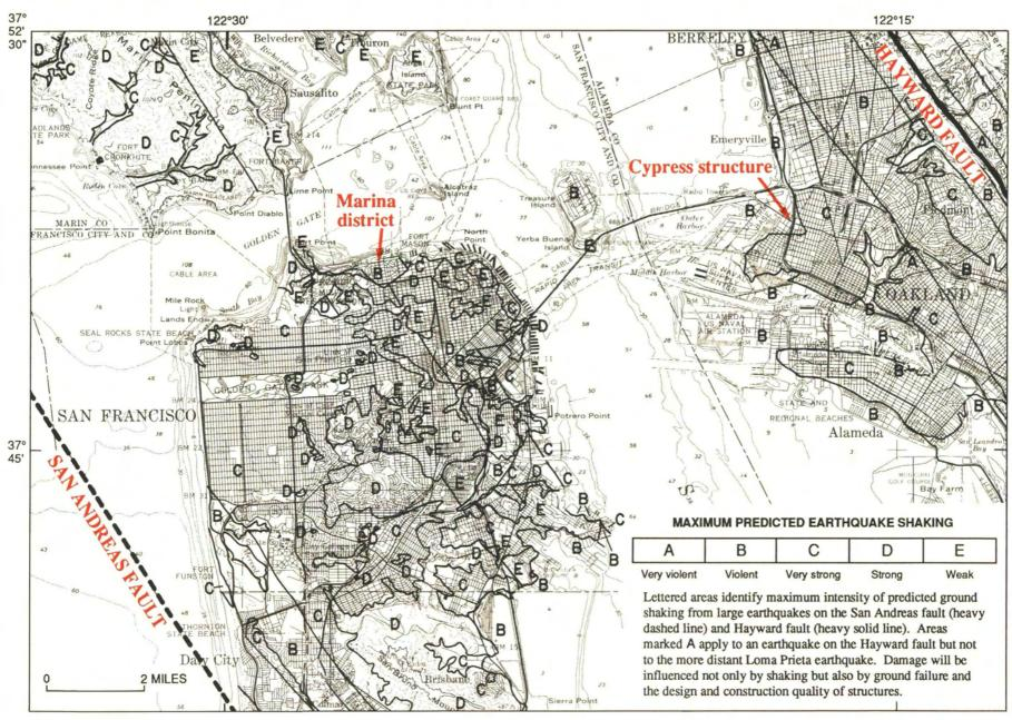
Much of the potential for damage from such earthquakes as the Loma Prieta event had been mapped as early as 1975, the release date of the map (U.S. Geological Survey Miscellaneous Field Studies Map MF-709) from which this illustration was
