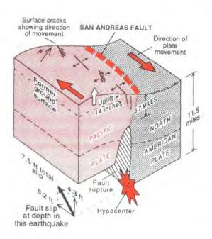
Changes in elevation and horizontal strain measured along the surface of the Earth after the Loma Prieta earthquake show that the Pacific plate moved 6.2 feet to the northwest and 4.3 feet upward over the North American plate. This motion was not observed along a single fault break at the surface but occurred in a complex series of cracks and fractures. The upward motion is related to deformation of the plate boundary at a bend in the San Andreas fault.
