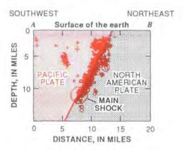
When the locations of the aftershocks are plotted on a vertical cross section oriented from southwest to northeast across the San Andreas fault, the fault is shown to dip 70 degrees to the southwest. The origin of the mainshock is the point where fault slip originated, from which it propagated upward and laterally both to the northwest and to the southeast.
